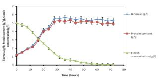
Figure 2. Time course of microbial biomass protein production and starch hydrolysis by *Candida utilis* NOY 1. All the experiments were carried out at 30°C, pH 5 and 150 rpm with 5g/L of starch. Fermentation was led 72 hours. Error bars show standard deviation among three observations. Values are means of triplicates  $\pm$  S.D. (Standard Deviation). The protein content is given in g of protein per 10 g of dried biomass.
