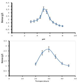
Figure 1. Effect of pH (a) and temperature (b) on the production of yeast biomass of *Candida utilis* NOY 1.
